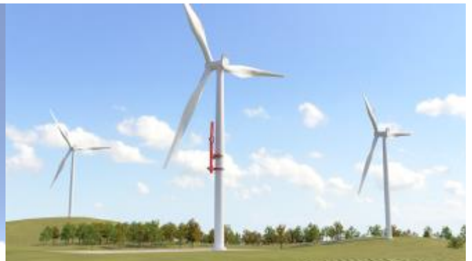
The WTM 100 ascends to elevation just below the turbine
